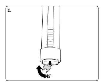
To remove the cups, move the quick release to the right.
