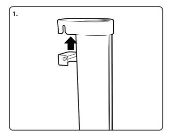
To transport the cup stacker (Item 1), lift off the bracket.
